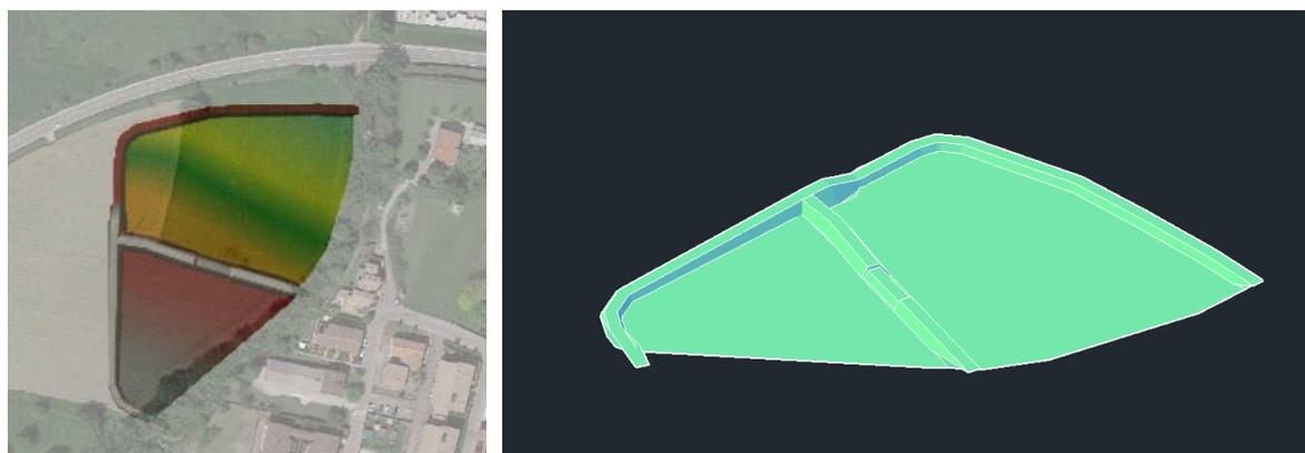
FIGURA 4-2 – RIO ENZOLA, MODELLO DIGITALE DEL TERRENO DELLE CASSE D'ESPANSIONE
